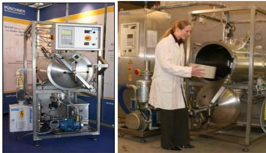
Figure 3. Members of the family  $\mu$ WaveVacxx50 from left to right -  $\mu$ WaveVac0150-1c with 1kW/2450MHz and  $\mu$ WaveVac0650 with 6kW/2450MHz.
