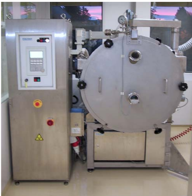
Figure 3. Microwave Disk Dryer for combined Air Circulation and Vacuum Mode µWaveVac0209
