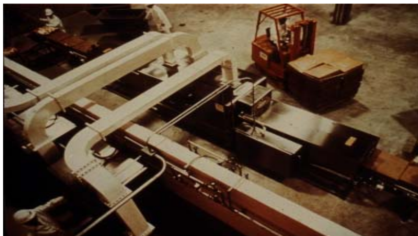
Fig. 7 Continuous microwave meat tempering system (Courtesy of Selo-Bollans Ltd)
