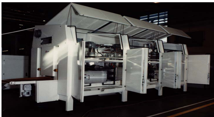
Fig. 8 Microwave puffing system for snack foods
