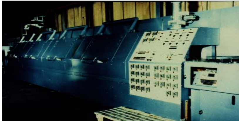
Fig. 9 Modular microwave pre-heater for rubber vulcanisation (Courtesy of Microwave Heating Ltd)
