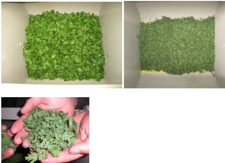
Figure 11. Drying of 10 kg basil in 40min using a combined microwave fluidized bed dryer under vacuum
