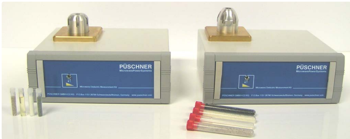
Fig. 1. Dielectric Kit for Vials (DKV) in two formats (standard vials of 1ml and 8 ml)
