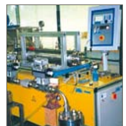
High Pressure Flow Heater of thermochemical Conversion of organic Compositions (250bar/350°C)
