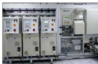
Full automated Multi-Batch Microwave System for drying Filter Cake down to < 0.1% Moisture Content
